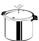
8. Assemble the three-piece pressure regulator to register the desired canning pressure (see page 4 for assembly instructions). See specific canning recipe to determine how many pounds of pressure to use.
